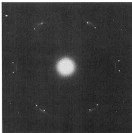
Figure 1. Electron diffraction pattern from a four-layer film of 65OBC at 62.0°C.
